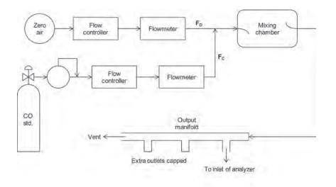
Figure 1. Dilution method for calibration of CO analyzers.
