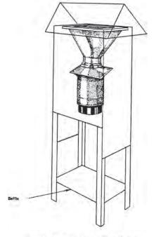
Figure 1. High-volume sampler in shelter.
