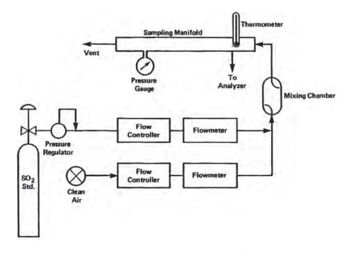
Figure 2. Calibration system using a compressed gas standard.
