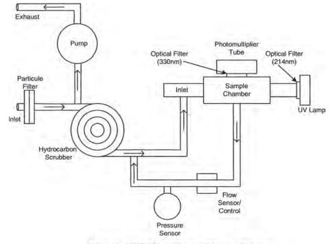
Figure 1. UVF SO2 analyzer schematic diagram.
