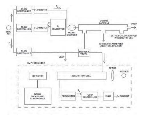
Figure 3. Schematic diagram of a typical UV photometric calibration system (Option 1).
