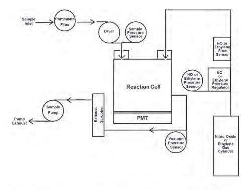
Figure 1. Gas-phase chemiluminescence analyzer schematic diagram, where PMT means photomultiplier tube.
